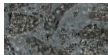
bocciardato / bush-hammered / gestockt
