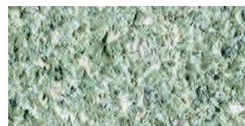
bocciardato / bush-hammered / gestockt
